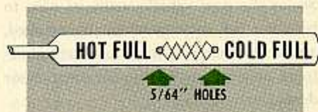
Fig. 3—By drilling two holes in dipstick, you make a sure thing of transmission oil-check.
