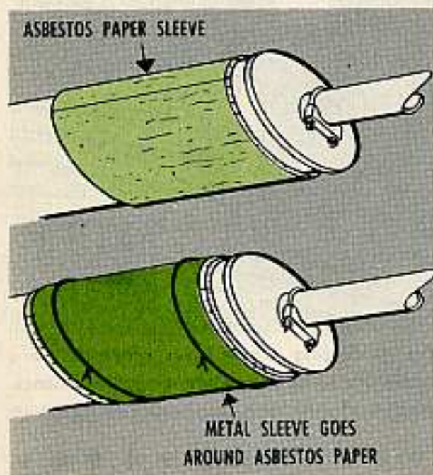
Fig. 4—Nothin' subs for a good muffler, but here's another patch that'll work in a pinch.
