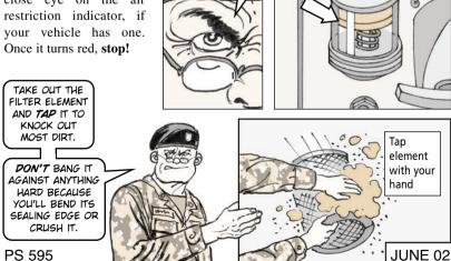
If your vehicle does not have an air restriction indicator, your engine will let you know when the element is clogged. You'll notice poor acceleration, lower power output or heavy black smoke from the exhaust.
