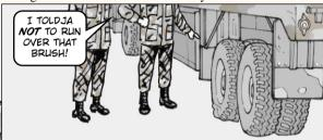
Take it easy moving over rocky, rough terrain. The sidewalls of radial tires are thinner than those of bias tires, and rocks cut them to ribbons. Wheeled construction and material handling equipment are especially prone to tire damage because the mission often requires them to work where the going is rough.
