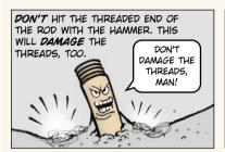
USE A DRIVING BOLT ON THE TOP SECTION AND MAKE SURE IT'S TIGHT. A LOOSE BOLT WILL BREAK OFF.
