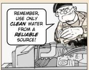
"WHILE YOU'RE ADDING COOLANT, TAKE A CLOSE LOOK AT THE RADIATOR CAP. MAKE SURE IT IS IN TOPNOTCH CONDITION AND IS THE RIGHT CAP FOR YOUR ENGINE. CHECK THE PRESSURE RATING ON THE CAP WITH THAT LISTED IN YOUR TM."
