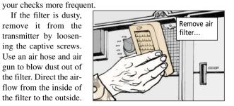
Don't use the air hose unless you have an air gun, NSN 4940-00-333-5541, to attach to it. The air gun limits the outlet pressure to 30 psi, a safe level that won't damage the filter or injure you.
