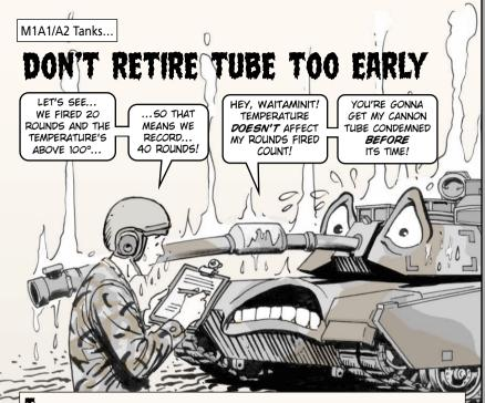
The M256 cannon tube on your M1A1/A2 tank isn't cheap, crewmen, so don't replace it before you have to. The safe service life of the M256 cannon tube is 1,500 equivalent full charge (EFC) rounds. For some cannon tubes, when the ammunition's ambient temperature rises to 100°F or higher, the EFC count increases from one to two for each round fired.
