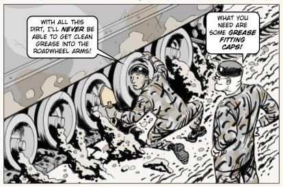
Getting all the dirt, mud, and sand off your combat vehicle's grease fittings before lubing is important, crewmen. Using a dirty grease fitting forces dirt and sand in along with the grease. Contaminated lube not only won't do its job, but it can damage bearings and other components.
