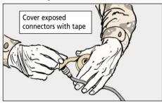
Plugs should be dried before inserting them into equipment jacks. Excessive moisture or dew should be removed from antenna connectors to prevent arcing.
