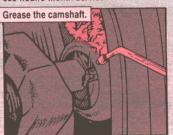
If you neglect 'em, the shafts will bind usually with the brakes on. Then the brakes drag, the linings glaze, and you may have a tire fire!
