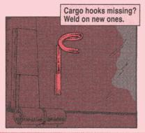
Remember, too, that those hooks won't stand the strain of a mechanical rope tightener. They'll snap off.
