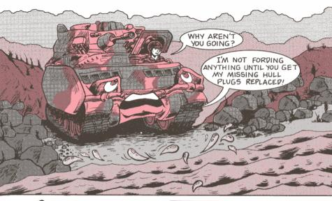
Grewmen, you've got to make sure the hull drain plugs on your Bradley are closed right and tight before operation.
