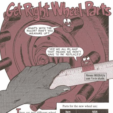
here are two different wheel assemblies for M939A2-series trucks, even though Fig 157 of TM 9-2320-272-20P shows only one.
