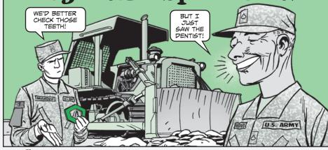
Construction operations cause the drive sprocket teeth on your dozer to wear down. Over time, enough wear can let the dozer's track jump right off the sprocket!
