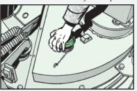
**2.** Remove the reservoir dipstick from the filler neck. Wipe it off with a clean cloth and reinsert it.
