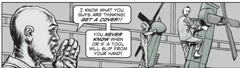
Mechanics, the last thing you need is to drop a tool on an uncovered Black Hawk or AH-64 stabilator.
