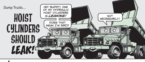
t's no secret that hydraulic hoist cylinders on M929- and M930-series dump trucks are known to leak. Some leak just a little, others leak a little more. Matter of fact, they're supposed to!
