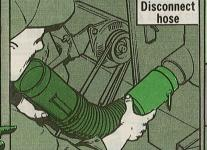
2. Open the engine access panel (lower panel only if you have the split panels) and pass the open end of the heater flexible hose through the
