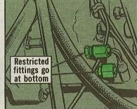
Another place where restricted fittings will really louse up the works is the 3rd and 4th oil scavenge ports on the gear box of a T-53 engine. A restricted fitting will give you a bearing failure in a metter of minutes.
