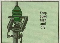
Cracked? Replace it. Eyeball the moisture seal, too. Remove the bowl once in a while and wipe it dry. Then put a light coat of silicone on both sides of both gaskets. An 8-oz tube is NSN 6850-00-880-7616
