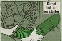
generator belt opening so hot air from the hose will hit the starter and thaw it out.
