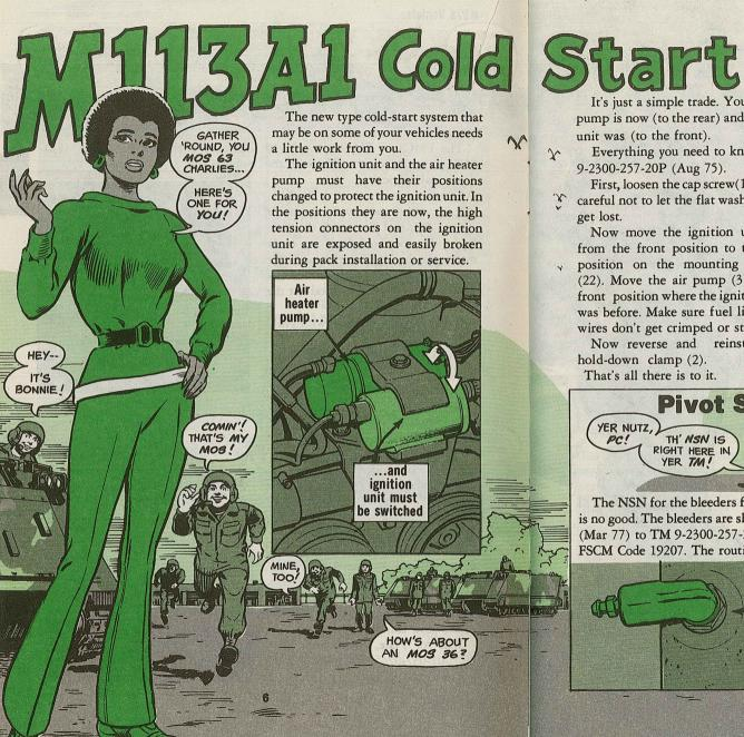
It's just a simple trade. You put the ignition unit where the air heater pump is now (to the rear) and put the air heater pump where the ignition unit was (to the front).
