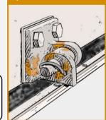
Bolts, clamps, nuts, and screws should be checked regularly for looseness.
