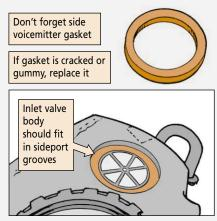
**New nosecup valve seat and new inlet valve:** NSN 4240-01-496-2844 brings 10 new valve seat assemblies that snap into place. Instructions come with the assemblies. NSN 4820-01-509-5498 is the new NSN for the inlet valve body.
