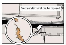
Mechanics, a new PMCS check is being added to the -20-2-1 TMs for the M1A1, M1A2 and M1A2 SEP. It requires checking for the cracks during semi-annual services. Make a note until the TMs are changed.
