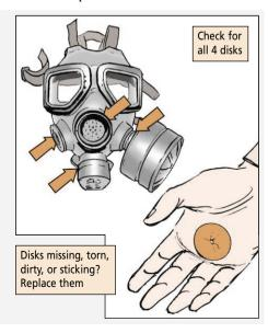
Outlet valve cover: Take it off and check for dirt. Don't forget to check under the disk. Wipe out any dirt with a clean, lint-free cloth. Make sure the valve cover and disk are not damaged. If the outlet valve disk is damaged, your mask won't have a good seal. In the field, check the cover for looseness.
