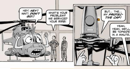
Mechanics, a loose or danging protective cap for the coolant fill port on your Kiowa Warrior's mast mounted sight (MMS) could mean trouble later.
