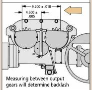
If the backlash is out of tolerance, they'll remove the center bottom cover and add a shim between the backlash gear and the gasket as shown on Page 13-22 of the -34-2 TM.
