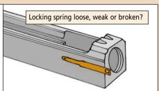
**Timing nut.** If the timing nut can be easily turned with one finger or it doesn't click as you move it, the nut's spring is too weak and it won't hold timing. Get the spring replaced.
