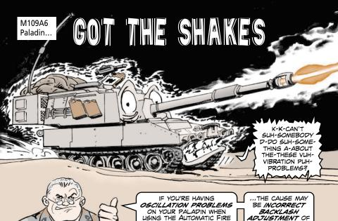
Have your mechanic notify DS/GS maintenance about the problem. They'll determine if the gear box has the correct backlash by measuring the traversing output gears as shown on Page 13-31 of TM 9-2350-314-34-2.
