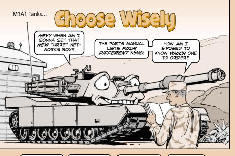
THERE ARE SEVERAL DIFFERENT CONFIGURATIONS OF MIAI TANKS OUT THERE. AND EACH ONE OF THEM USES A **DIFFERENT** TURRET NETWORKS BOX (TNB). SO HOW DO YOU MECHANICS KNOW THE RIGHT TNB TO USE WITH A PARTICULAR TANK? THERE ARE
