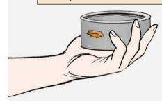
Canister: It's OK for the canister to have dents as long as they're no deeper than 1/4 inch. If they're deeper or cross a seam or threads, it's time for a new canister.
