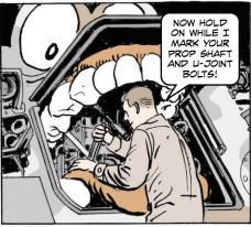
Ine of the most important things you crewmen and mechanics can do is check for loose or missing propeller shaft and U-joint bolts on M113 carriers.
