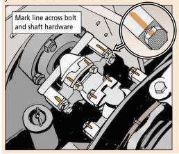
That makes it easy for crewmen to double-check them during PMCS. If the marks don't line up, the bolt has loosened.
