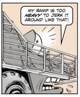
With the addition of slat armor, the ramp on your Stryker becomes a real heavy-weight. That means you have to be even more careful than normal when raising and lowering the ramp.
