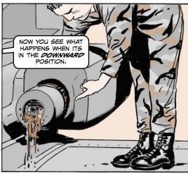
Mechanics, it's important how your AH-64's nose gearbox filler cap is positioned. Make sure the cap is turned to the aft and upward position to protect against strikes on the tab from birds or branches.
