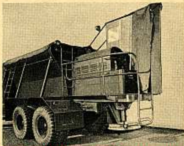
CINDER SPREADER, FEDERAL TRUCK, MADE BY UNIVORYOR-SAUGHMAN MFG CO. IT HAS A 5-TON HOPPER (COAL BODY, SELF UNLOADING AND THE SPREADER ATTACHMENT IS HOME MADE.)
