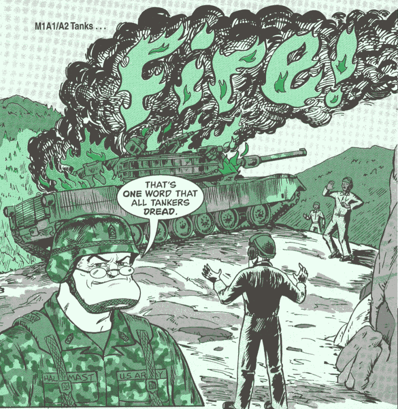
NBC filters can overheat and burn
