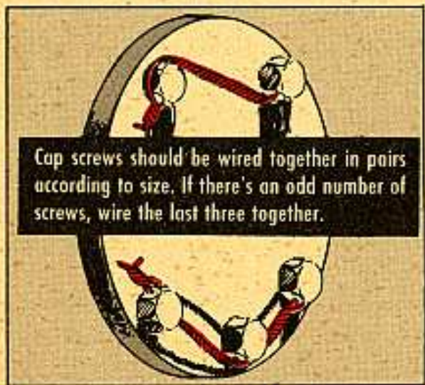
In the two cases above the safety wire goes over the head while in the two cases below the safety wire goes around the head. Safety methods shown are for right hand threads—left hand opposite.
