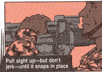
Grab sight just in front of right bumper with thumb just under sight. That gives sight more support
