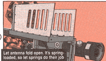
Lay antenna over until it stops moving. If you jerk it out, eventually it breaks. That's a depot fix
