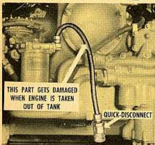
Fig. 1—Some tanks have the main fuel-line on engine with quick-disconnect like this.
