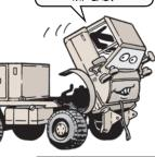
It's real easy to damage the engine's throttle linkage and mounting bracket when you tilt or lower the small emplacement excavator's cab.
