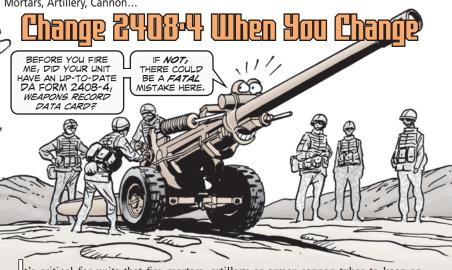
It's critical for units that fire mortars, artillery or armor cannon tubes to keep an accurate DA Form 2408-4, Weapons Record Data Card, for each weapon. Without an up-to-date card, the weapon could be fired after its cannon tube should have been replaced. That could be a fatal mistake.
