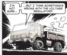
Are the instrument panel lights on your FMTV flashing on and off? If so, you could have a problem with the voltage regulator found on the 260-AMP alternator.
