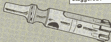
Bolt ring gaps staggered?
