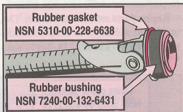
For cold weather use gasket NSN 5330-01-271-7621
