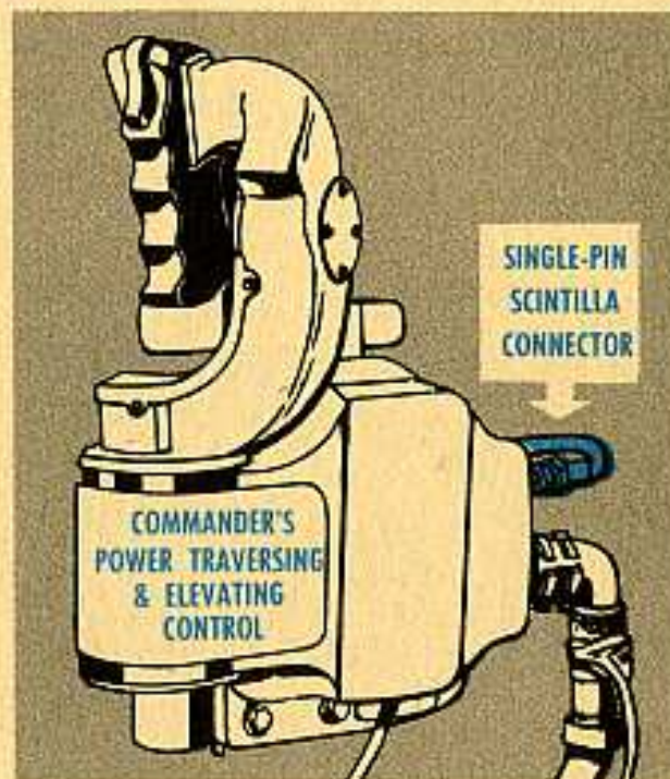
Fig. 1—By disconnecting this single-pin Scintilla-connector, the commander will not be able to override while the gunner's in manual control—meaning no stripped gears.
