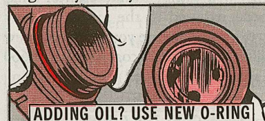
ADDING OIL? USE NEW O-RING!
