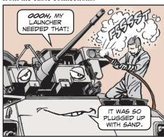
Seal sand out of the launcher with the dust curtain, NSN 1005-01-126-7797. Keep the curtain closed whenever the launcher isn't being used. If the studs that hold the curtain in place have disappeared, order more with NSN 5315-00-174-2882. While you're waiting for the studs to arrive, use hook-and-pile tape, NSN 8315-01-470-8453, to hold the curtain in place.
