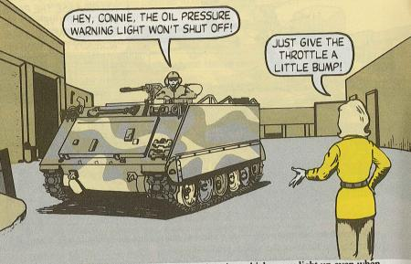
The oil pressure warning light on M113-series vehicles may light up even when the engine oil pressure is OK.
