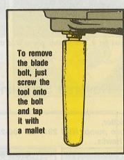
The bolt and tool slip through the grip and blade holes without damaging either.
