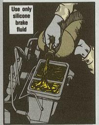
Keep those HMMWV's humming with the fluid's purple. Any other fluid gums up the equalizer valve and master cylinder Too much grease is as bad as too little and jells in the system. This makes for a big job to take the brake system apart and clean it.
