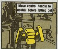
So, move your power control handle to neutral before you let go of it—every time. In addition, never release the control handle palm switch while traversing the turret. If you do, you could cause wear or damage to the magnetic brake and the pin lock. **JAN 88**
