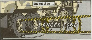
For that long reach, you'll need a tire pressure gage, NSN 4910-00-441-8685. It comes with a 10-ft hose, a quick-disconnect coupling and two coupler adapters. Hook it to the air supply hose with a straight pipe-to-tube adapter, NSN 4730-00-391-3771. It's in the No. 1 Common shop set's brass fitting kit.
