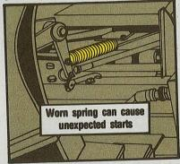
The gearshift is spring-loaded so that you must push the shifter to START to crank up the engine. The shifter is then pulled back to NEUTRAL by the spring.
