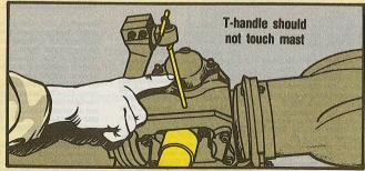
If the work aid touches the mast, back it out some. Otherwise, it's sure to damage the mast when you remove the rotor assembly.
