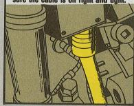
Check the ground wire from the battery to the hull. Make sure the ground cable is tight.
