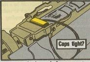
on the monitoring set's four connectors. Uncovered connectors are wide open to dirt, which prevents good connections and causes pin damage.
