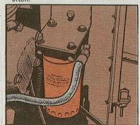
Two water filters are available: PN 31007441365C1 for new coolant. PN 31007442816C1 for old
