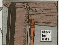
Hold one! That hoist cylinder must have a thin film of oil on its polished surface.
