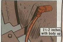
BLEEDING—Look for slow or unsteady hydraulic cylinder action. If the oil in the reservoir is low—or if air got into the hydraulic system the cylinder may need bleeding.
