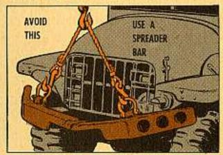
Besides hitching the tow-bar to the towed vehicle's front-axle, you've got to rely on the lifting hooks to take 'er off the ground. You can do this by clamping a wire rope across the hooks, and picking the truck up by the rope. That way you'll raise the vehicle and not the devil.
