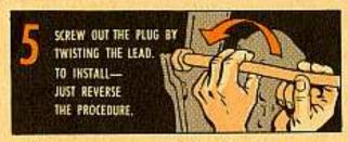
Take care to avoid side pressure keeping the wrench in line with the plug as y'loosen it—and those heli-coil inserts'll stay put.
