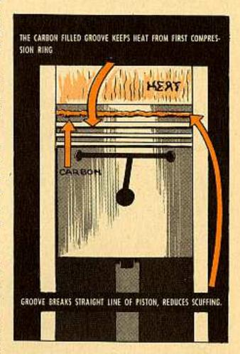
the life of the fire ring. At the same time, by breaking the straight side of the piston, this groove tends to reduce the tendency to scuffing.
