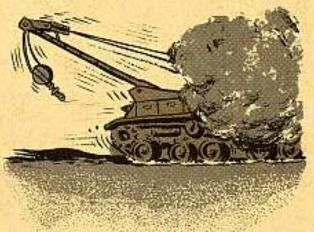
And for goshsakes, don't attempt to make a lift from the boom until it's all the way up and the boom-support staycables are tight. If you do, you use your lift to build up excess pressure in the lines, and they may carry away.
