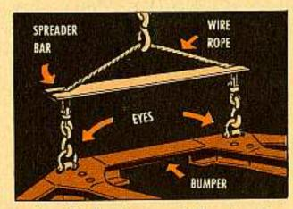
a spreader-bar to spread the rope. Else, you'll bend the eyes and bumper.)
