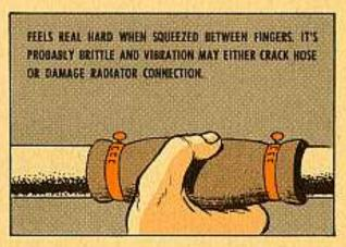
If it feels real soft, it's probably rotting out, This can fill the cooling system with small particles of rubber which can clog and overheat the engine.
