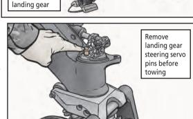
Remember to remove the landing gear steering servo pins before towing. That lets the landing gear turn freely. If the pins are left in, the servo and landing gear get damaged. And it's so easy to forget the pins. Just make sure you reinstall the pins before takeoff.
