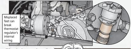
When that happens, the cooling fan will no longer run at high speed when extra cooling is needed. The engine can overheat. Even if you manage to catch the problem before losing an engine, a new thermostat regulator will set your unit back nearly \$8,000.
