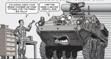
Mechanics, take extra care when loosening or tightening the exhaust air hose on the Stryker's brake chambers. Return line elbow pipe fittings are ending up bent or cracked. That makes a brake chamber unserviceable and that means an NMC Stryker.
