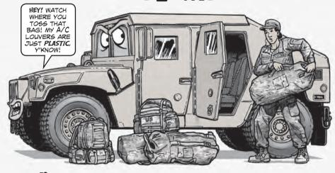
BEFORE YOU HIT THE ROAD, CHECK WHERE BAGS AND GEAR ARE PILED IN THE BACKSEAT. IF YOUR HMMWV IS EQUIPPED WITH AIR CONDITIONING VENTS ON THE BACKSEAT CONSOLE, YOU MAY NEED TO RE-ARRANGE THINGS.
