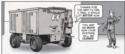
The new filters, which are completely interchangeable with the old ones, will be added to the next TM updates for the H-60, AH-64 and AGPU. Until then, order the new filters from this list:
