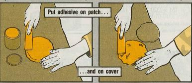
Let the adhesive dry (about an hour or so), then apply a second coat. When the adhesive is tacky (10-15 minutes), center the patch over the damage.
