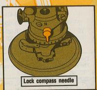
Instead, first turn down all three leveling screws-at the same timeuntil the M2 is tight against its base. Then loosen the screws-together-**SEP 87**  a quarter turn. Lock the compass needle. Cover the orienting knobs and level vials. Position the azimuth knob over the notation pad. The procedure's on Pages 62 through 65 of TM 9-1290-262-10.
