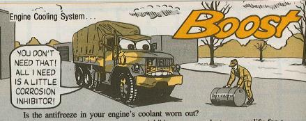
If the only problem is worn-out rust inhibitor, your coolant may qualify for a dose of inhibitor, corrosion, liquid cooling system, NSN 6850-00-753-4967. It's listed in Para 2b(3), TB 750-651, Use of Antifreeze Solutions and Cleaning Com-
