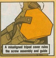
· Always turn all three leveling screws at the same time. Turning one or two screws at a time can bend the spring plate—a general support fix.
