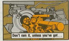
...at least 925 PSI on the hydraulic pump pressure gage
