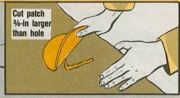
Spread adhesive on the back of the patch and on the cover around the damage.
