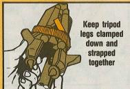
could be broken or bent by a heavy object—like someone's foot. If the tripod cover's off-center, that heavy object could ruin the screw assembly and guide that hold the M2 on the tripod. bend the spring plate, too. **SEP 87**
