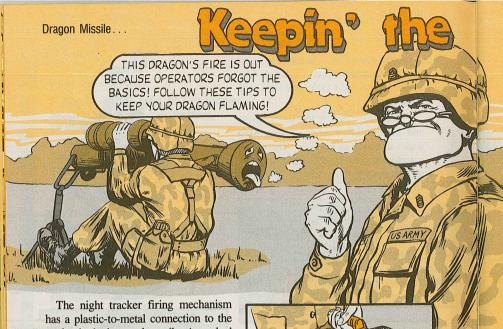
tracker body that cracks easily. A cracked mechanism makes the night tracker useless. Protect the firing mechanism with careful handling. When you lift the night tracker out of its bag by the firing
