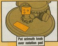
Remember, moisture causes corrosion- and you can't read corroded scales! So always wipe the M2 completely dry before you stow it.
