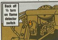
adjusting. Just turn the adjustment screw out till the blower goes off, then back it Voltage to the igniter is important— off ½ turn more. Make this adjustment
