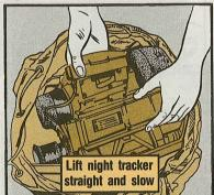
mechanism, don't jerk it up. Straight up and slow is the best way. Once the night tracker's out, immediately switch hands to the carrying handle. And use the carry-
