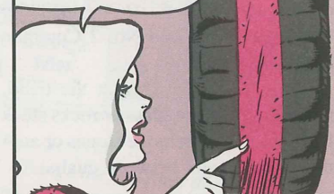
You get fast wear in the center... while the edges wear slowly
