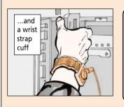
NSN 4940-01-253-5368 BRINGS A FIELD SERVICE KIT WHICH HAS THREE BARRIER BAGS, TWO WRIST STRAPS, ONE GROUNDING CORD AND A WORK SURFACE MAT.
