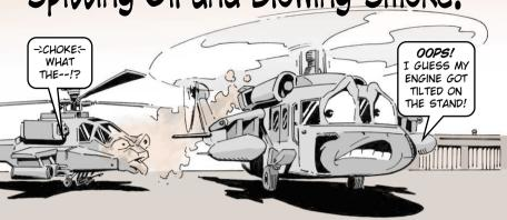
You might think, crewmen, that spitting oil and blowing smoke from a reinstalled engine means pulling it again to have AVIM replace a bad seal. But, the problem may be that you tilted the engine when you removed it for AVIM repair or when you re-installed it after repair.
