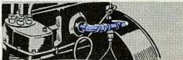
Donaldson valve—to stop crankcase pressure build up, keep its inner workings clear.
