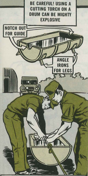
Some outfits like this homemade rig—a half-drum with a hook on each end. This tank is slid along the cable while one guy brushes off the dirt and the other sloshes on oil.
