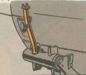
Traversing lock bent, broken, missing. Spacer sleeve missing
