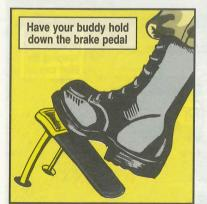
Open the bleeder valve. Watch the fluid as it flows thru the tube. When you no longer see air bubbles, or when the flow stops, tighten the valve and holler Whoa!
