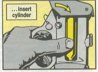
Watch it, tho. The cylinder should fit in the hole snug. If the cylinder wiggles, something's wrong with your M11. Turn it in.
