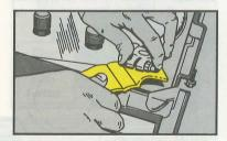
Push the terminal clamps all the way down on the battery posts and tighten them.
