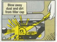
use an air hose to clean the area around the filler cap. Of course, you always wear goggles when you clean with compressed air. A LITTLE HOUSEKEEPING
