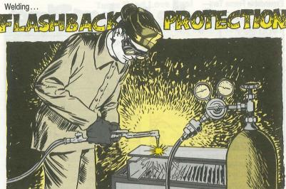
flashback in a welding hose can cause an explosion or fire in the regulators or tanks.
