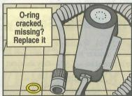
Make sure an O-ring is in a connector. If the O-ring is cracked or missing, get it replaced. Without an O-ring, moisture will get inside the connector and short out your commo equipment.
