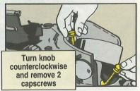
Turn the crosslevel knob clockwise as far as it will go. Remove the other two screws and washers.
