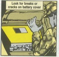
Make sure the batteries are seated and clamped down.
