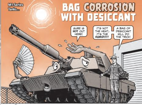
Crewmen, there's nothing much worse than humidity in the ammo compartment for your M1-series tank's onboard ammo. That gives rust and corrosion a foothold. Whether your tank stays uploaded all the time or only during exercises, the risk is always there.
