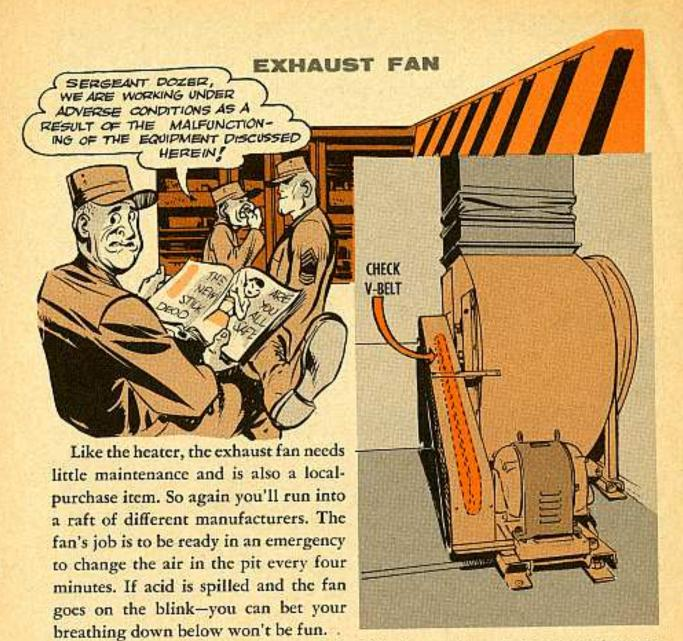
The motor and fan bearings and the V-belt are the only items you have to check out come maintenance time. Most of the fans have sealed-for-life bearings, but if yours is the type that requires lube—see that it gets lubed. Even though it's a light-duty fan, don't use a light-duty oil like the common household or sewing machine oil. Use at least 10-weight oil.
