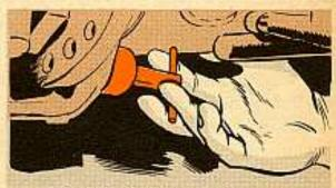
and the lock pin in the steering gear box.
