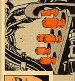
7. Leaving the turnet power ON, bleed the remaining elevating system lines by using the bleeder valves on the anchor plate located on the forward turnet wall below the elevating hand pump. Loosen each plug (here you'll use a \$\frac{1}{2}\ellipse in wrench), bleed the air, retighten the plug and go on to the next one.
