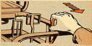
Now when you come to engage the main transmission, you'll have to squeeze the clutch pedal down by hand...
