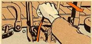
Then shift the vehicle into low-rangethat is, bring your auxiliary shift lever to the back position.
