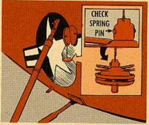
But a good crewman goes one step further and looks carefully at the bottom of the filler cap itself—since that spring pin hole in the cap has been known to wear itself oversize and let the whole works drop down into the fuel cell. Which leads to the devil's own job getting 'em out again.
