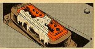
Water gets into the receptacle and around the contacts by condensation and from tunnel No. 3. There's no sure way of keeping water out of tunnel No. 3. It gets there by condensation. And water can run into the tunnel in bad weather if the tunnel's been taken off and put back on a good many times.
