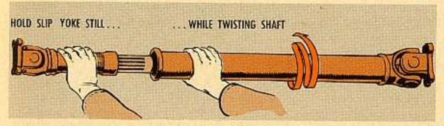
If your inspectors aren't holding that slip yoke stationary when checking the shaft, they can get a false impression. They'll get play from the power train or from a worn universal joint. That'll give the impression of too loose a shaft.
