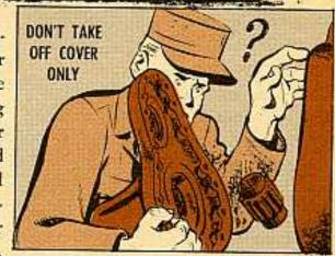
And, what's worse, you may be tempted to put it back... the wrong way. Y'see, the final drive pinion is counterbored at the end that's toward the transmission, so's the final drive in-put shaft will fit into it.
