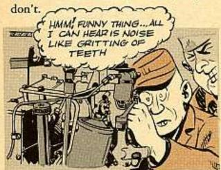
On your M42's after serial number 1385 and on your M41A1's after serial number 3589, a new type of fuel-line quick-disconnect coupler assembly (FSN 2910-620-0932) was put in. When connecting or disconnecting this coupler, you'll hear that metallic scratchy noise. Don't let it worry you you want it there.
