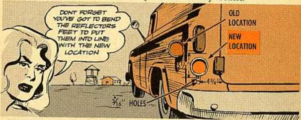
First, take the two tapping screws out of each reflector—but don't throw 'em away. Weld or lead shut the gapping holes left from the removal of the screws, Smooth off the filling, and prime and paint—like it says in TM 9-2851.
