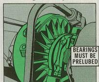
drains away, dries up or hardens on the bearings. Since you don't idle the set, those 2000 operating RPM's hit and heat the unlubed bearings as soon as the engine starts. This is guaranteed to burn 'em up!
