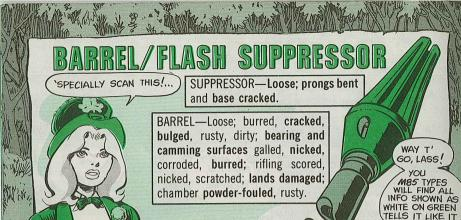
Here's the best way to beat the barrel rust and carbon hex: After firing, clean the bore with RBC, wipe dry . . . then add a light coat of LSA. Just before firing, run a patch thru a couple of times. The bore should be dry to stop carbon build up and stop the big bang caused by the increased chamber pressure due to the oil in the bore.
