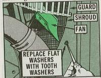
Replace the 4 non-locking flat washers MS27183-10—item 2, fig 46, TM 5-6115-545-24P(Jun 73)—with ¼-in ID internal-external tooth washer MS45904-68(96906) NSN
