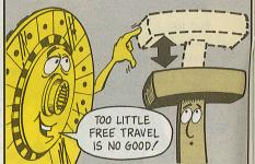
Free travel moves the clutch throwout bearings toward the clutch release levers. The bearing starts spinning as soon as the bearing touches the levers.
