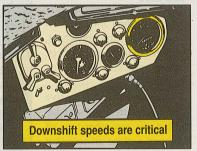
You don't go from 2-3 range to 1-2 at 35 MPH, for example. You could have more transmission parts flying than there are hornets in a nest.
