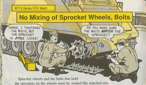
Mixing the two sizes of bolts with the two types of sprocket wheels causes equipment damage and crew injury.
