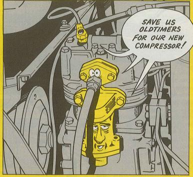
It's impossible to make ends meet when you put a new air compressor on a 2 1/2- or 5-ton truck unless you save some of the parts from the old compressor. Some mechanics turn in compressor, NSN 2530-00-863-3155, with the accessory parts still attached. They think they'll get all new stuff.
