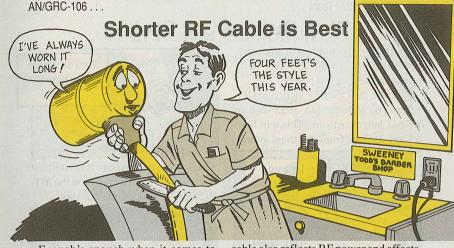
Enough's enough when it comes to the length of the CX-10171 electrical lead between your antenna and radio set.
