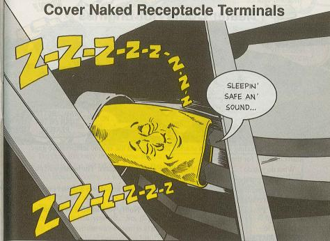
Naked cable terminals on this 5-tonner's slave receptacle are trouble waiting to happen. If anything metal, like a wrench, touches the bare terminals, it will cause a short that can start a fire.
