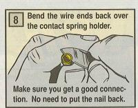
After step 5, if the wire's too short to let you strip 1/4-in off each end, replace it with a 13 1/4-in length of wire, NSN 6145-01-010-7014, that's had 1/4-in of insulation stripped from each end.
