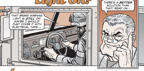
Something is wrong when the brake warning light stays on (no kidding!). But before you replace any parts, make sure you bleed the vehicle's brake lines.
