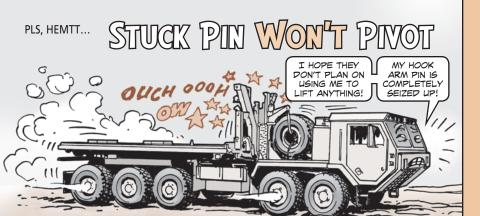
Drivers, the load handling system (LHS) hook arm on your PLS or HEMTT won't be grabbing many loads if you don't keep its pin, NSN 5315-01-361-2721, lubed. Some of those pins are going unlubed so long that they have to be removed with a
