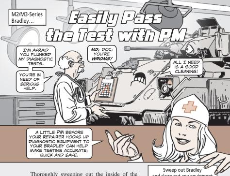
Thoroughly sweeping out the inside of the Bradley should be your first step. Be especially careful to clean underneath the gunner's seat where the main diagnostic connections are. Dirt can foul the connectors, which hurts the accuracy of the tests.
