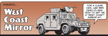
The mirror in this kit is larger than the older-style side view mirror, and also has a convex, wide-angle view area that improves the driver's field of view.
