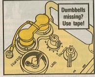
If you find transmissions fading or gone, even tho you still get good reception, try a new battery before sending the set off for maintenance. Remember, it takes more juice to transmit than to receive.
