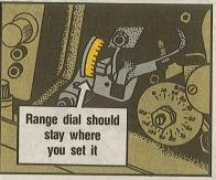
2. Eyeball the range adjustment. Make sure it's still where you set it. Chances are it won't go out on its own. Try to keep adjustments to a minimum. Too much fiddling can lead to failure. That leads to bad readings.
