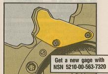
Remember! Gages are used to measure wear only on sprockets without wear mark indicators on them. TM 9-2350-253-20-1 gives the full procedure. **SEP 84**
