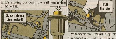
disconnect pin, make sure the retaining mechanism (spring-loaded balls) is holding the pin firmly. Just pull on the pin. If it comes out, clean it or replace it with a new pin.
