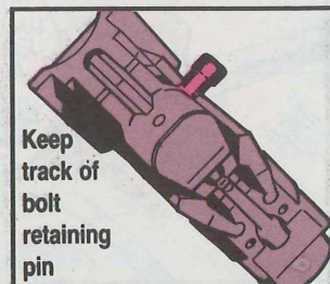
Ball lock should be firmly seated in the detent knob notch
