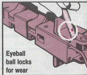
Ball lock should be firmly seated in the detent knob notch
