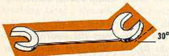
Fig. 4—This tool eases engine-assembly removal on tractor-truck (Model H-542-211).
