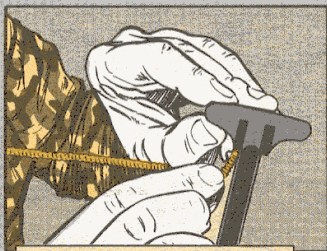
Use a rag, pipe cleaner and CLP to clean the charging handle
