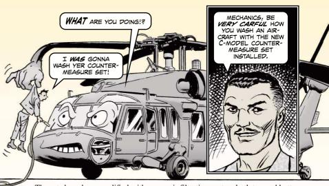
The sets have been modified with a new air filtration system both top and bottom that cannot take wash water.
