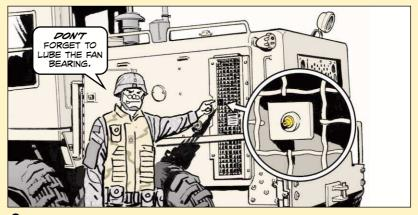
One small PM tip that really matters on this road grader is the grease fitting for the fan bearing.
