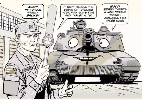
Tightening the king and thrust nuts during a tank's gun tube replacement requires a **minimum** of 1,000 lb-ft of torque.
