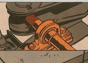
UNIVERSAL JOINTS—Damaged. broken: painted over so's there's no free 'n' easy movement. Pipe assembly broken, bent.
