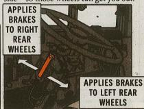
This's something to remember with your own car. Sometimes it'll get you off a slippery spot—when the rear wheel on one side is spinning. You apply your brakes very lightly to keep that wheel from spinning. Power will be transferred to the other side where the wheel is just sitting still. If you're careful-and lucky-it'll get you going.
