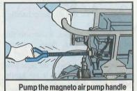
That's even more important on the new M3A4 because its handle slides out of-and cracks-its housing more easily than the old generator.
