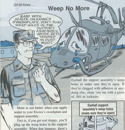
assembly. When that happens, there's no place for water inside the dust boot to escape.
