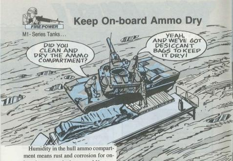
ment means rust and corrosion for onboard ammo, whether your M1 stays uploaded all the time or only during exercises.
