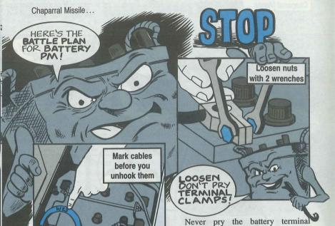
Lots of Chaparral launching station batteries are being killed because operators pry off and pound connectors onto terminals, let corrosion eat away connectors and terminals, and hook up batteries wrong. Declare war on poor battery PM with this battle plan.
