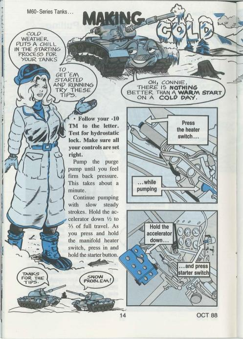
If the engine starts, keep pumping the purge pump with steady strokes, holding the manifold heater switch and the engine starter button until the tachometer reads 450–500 RPM.
