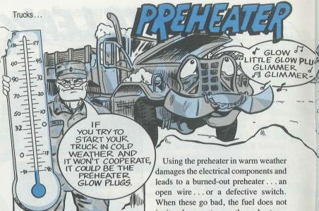
The manifold air preheater on some diesel and multifuel engines helps start those big engines in cold weather-32°F or below. But you shouldn't use it for quick starts when temperature's above 32°F. Or to prime a hard-starting engine when something else is wrong.
