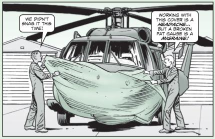
**M** echanics, putting on and taking off the Black Hawk nose cover is not that simple. Pay attention to the free air temperature (FAT) gauges when removing or installing the cover. Make sure the slots in the cover fit over the gauges.
