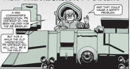
If the palm lever assembly (also known as the Cadillac) of the grip and gimbal assembly of the old handstation is installed in the new handstation, the turret or gun could move unexpectedly. That's a danger to your crew.
