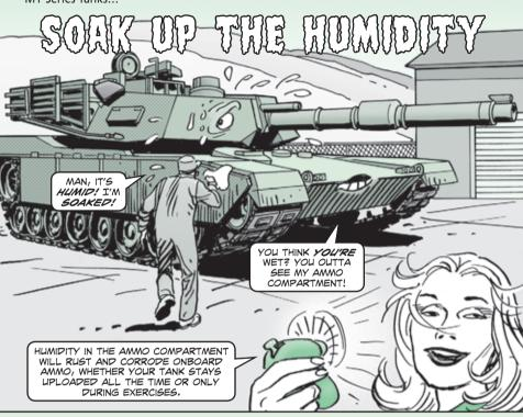
Sure, you can slow the damage by occasionally wiping away any condensation in the ammo compartment. But to really put the brakes to corrosion, you've got to stop moisture.
