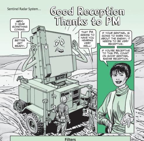
Clean filters give the Sentinel plenty of clean air to stay cool. Clogged filters lead to breakdowns like blown fuses in the high voltage bay. The Sentinel has eight filters (make that 10 for the newest version) and all the filters need to be cleaned at least weekly. In the desert, make that daily when you're operating. Remember, too, that filters will clog quicker after rain.
