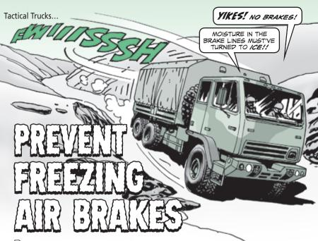
Drivers, moisture can build up in your truck's air brake system even in good weather. Over time, that moisture corrodes air lines, relief valves, check valves, and the air tanks, too.
