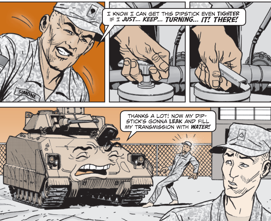
Too tight on T-handle will damage gasket
