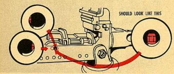
Don't fool around with your .50-cal machine gun if the outer lug on the barrel locking spring doesn't center in the hole on the receiver when you're headspacin' the weapon. Ask your Ordnance support for another gun and file a UER on the snafued weapon.
