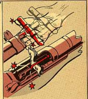
Bang the rod, and those shoulders on the handle will scrape the outside of the muzzle and scar it up and bang the rod end into the follower. Your 3.5 Rocket Launcher:
