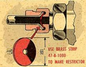
which tells field maintenance (or higher) how to install a restrictor in power-divider governor valve control, valve-to-power divider governor valve vacuum line. It'll govern engine speed when crane hydraulic pump is engaged and the power divider is disengaged. This MWO is a must.
