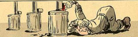
Now, comes the shot in the dark. Take your hot rod out of the flue and put it in the vaporizer, but turn your head away so your face isn't over the hole. Even though your head's turned away, you shouldn't have any trouble hitting that canyon-like hole. Finally, adjust your gasoline-adjustment valve to the kind of flame you want. Get familiar with TM 10-702 for details on your heater.
