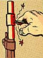
Never use a rod like this to take out a tight or frozen gas-cylinder lock-screw.
