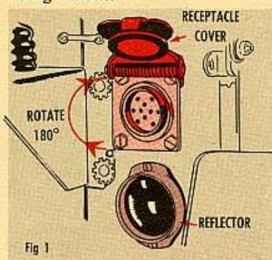
This means that when the cable is installed the cable end cover has to open back and downward—toward the reflector. In that position it bangs against the reflector, scratches and cracks it.
