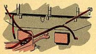
The other method is to straighten the air hose out and then give it a twist before you connect it to the truck.
