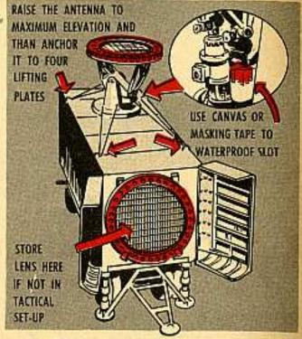
For M33 people who aren't involved in a tactical set-up, protecting the track antenna's lens in hurricane-like weather is a simple matter. They just remove the lens and store it inside the clamshell where it normally goes when the van's on the move.
