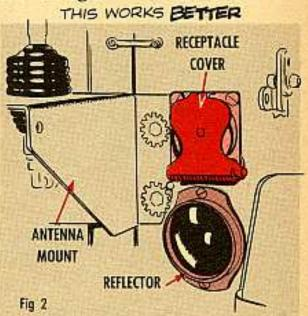
But we've found 'that rotating the receptacle 180 degrees (Fig 2) instead of 90 degrees clears everything up. Lets the cable end cover open out and upward — where it won't bump into anything.
