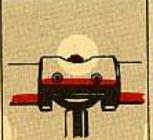
First, put rod together right. The stem is screwed through the beveled side until it comes out the other side of handle.
