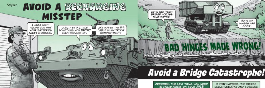
Mechanics, figuring out why a Stryker's batteries aren't charging can be tricky and time consuming. But you might save yourself some trouble by making the W4 cable inside the troop compartment one of your first checks.
