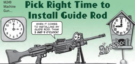
Soldiers are installing the M249 machine gun's guide rod assembly wrong. Eventually, that damages the receiver so much it must be replaced.
