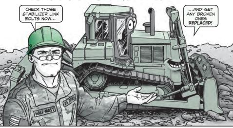
• perators, take a minute to eyeball the condition of the Grade 5 mounting bolts on your D7R II dozer's stabilizer link.
