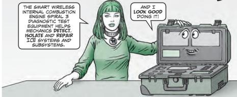
The SWICE SP 3 connects with the Maintenance Support Device version 3 (MSD-V3) and the equipment tested to perform standard voltage, current, resistance, pressure and rpms and capture digital diagnostic data.
