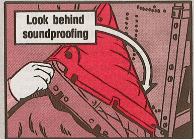
Check drain holes
