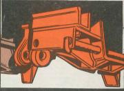
CUTTING EDGE-Worn, chewed up, bolts missing or loose.
