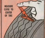
gage so its bar spans the tread. Press the plunger easy-like and take your reading when its tip touches the tread groove. Check the tread at 3 evenly-spaced points around the tire. If you have a reading of 2/32 inch at any point-it's time to demount it.
