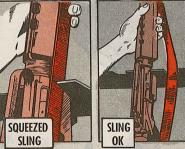
slots. Wears out the sling and destroys the rifle finish at the contact points.
