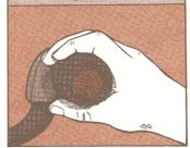
Look for dirt and sand in the connector and MGS jack. They cause a poor connection and bent pins.
