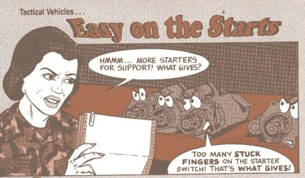
old weather is here and so are those itchy fingers that stay stuck on an engine's starter switch. All it takes is one finger stuck on the switch too long to burn out a good starter motor. When you try to start your truck engine, never keep the starter engaged for more than 10-15 seconds. Stop! Let the starter cool one minute. Try again.
