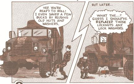
Once is enough for lock washers and locknuts. When your TM tells you to discard locking hardware, toss it.
