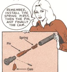
4. Use no oil when you assemble the mechanism, and dry off all parts before assembly.
