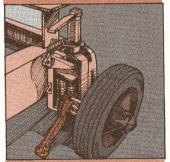
✓ Make sure the platform wheels and caster are lubed according to TM 55-1730-223-13 & -23P.
