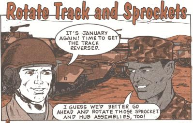
Unidelines now require that T158 track on M1-series tanks be reversed annually. That evens out shoe wear and makes the track last longer.
