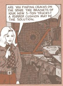
hat balloon tire on the new 5-ton has proven to be too much of a load for some brackets. The base cracks where the bracket mounts to the truck or where the bracket bolts to the base.
