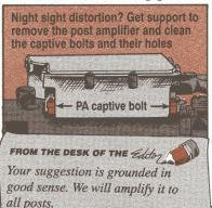
...we had support remove the post amplifier and clean out all the dirt and corrosion from the four captive bolts and their holes. Seems crud was preventing a good ground.
