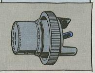
BATTERY CAP & HOUSING—Dirty, greasy, corroded or pitted contacts
