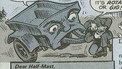
We get gigs because the lunettes of our M416 1/4-ton trailers are not free to be rotated by hand. This is blamed on rust, lack of lube, etc. After shining and greasing the tapered stem, we adjust the spring to the specs in our manual. This makes the lunette tight like a cork in a bottle.
