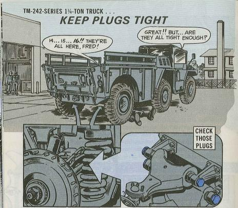
Goat when it's got all 16 of its front eyeball Fig 2-295, page 2-292, and Fig and rear suspension arm plugs—and 2-298, page 2-296, in TM 9-2320-242they're all tight.
