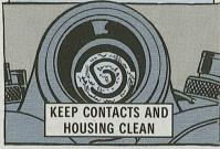
(TIPS: Keep contacts clean with a burnishing tool or crocus cloth. When you replace cap, line up the slot, push cap down, then turn knurled knob snug. When you back the cap out, wiggle it slowly. Saves busted caps and slots.)
