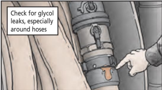
Check for glycol leaks, especially around hoses
