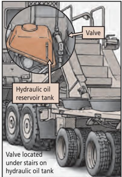
TM 9-2330-381-13 (Oct 09, w/Ch 1, Apr 15) shows what the valve's open position looks like. It's pretty simple. The hydraulic tank also has a label next to the valve, indicating the open position (handle down) and closed position (handle up).
