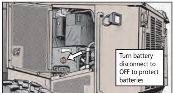
Turn battery disconnect to OFF to protect batteries
