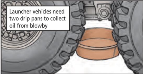
Launcher vehicles need two drip pans to collect oil from blowby
