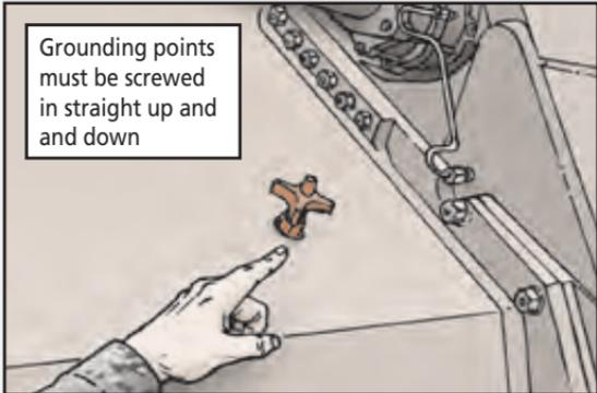
Grounding points must be screwed in straight up and down
