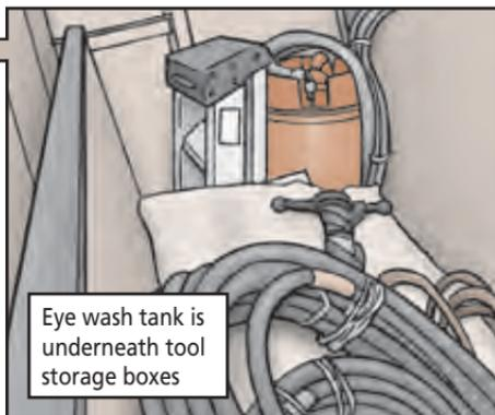
Eye wash tank is underneath tool storage boxes
