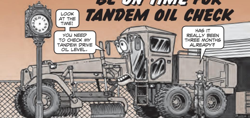
**O**perators, don't forget to check the tandem drive's oil level on your 120M road grader every three months or 500 miles, whichever comes first.
