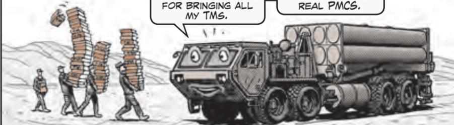
When THAAD is in the motor pool, we generally do a daily PMCS on the missile system and a weekly PMCS on the trucks. In the field, we do a complete PMCS on everything daily. PMCS always includes powering up the system and checking for faults.
