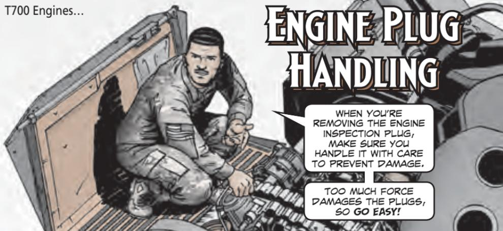
They, 15B engine mechanics! WP 0325 and WP 0331 of TM 1-2840-248-23&P (Jun 17) tell you how to remove and install the Apache and Black Hawk's engine inspection plugs, NSN 5365-01-091-4688 and 5365-01-106-9667, for borescoping.
