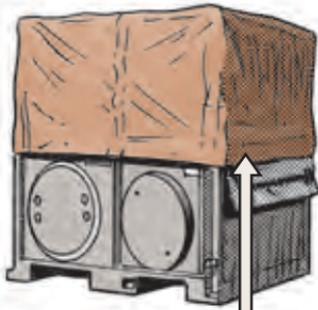
WHEN THE IECU'S NOT IN USE, PUT THE VINYL COVER OVER THE CONDENSER FAN TO KEEP DEBRIS FROM COLLECTING IN THE CONDENSER (TOP) SECTION. A DEBRIS-FREE IECU IS LESS LIKELY TO GET DAMAGED OR WORK POORLY.
