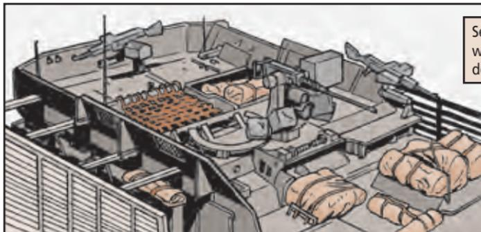
Secure gear to roof with nets and tie-down straps
