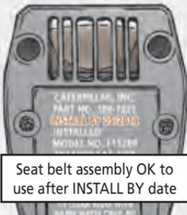
Seat belt assembly OK to use after **INSTALL BY** date
