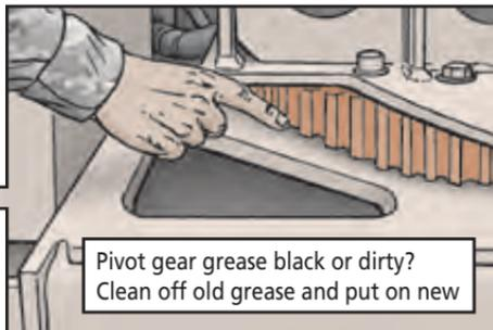
Pivot gear grease black or dirty? Clean off old grease and put on new
