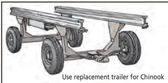
As you stated, there are no repair parts available for those trailers. So you'll need to order a substitute trailer instead. The replacement is **ground handling trailer**, NSN 1740-01-542-1099. Get ready for sticker shock, though. The trailer costs a little over \$11K. The manuals have limited repair parts and some of the parts interchange between trailers.
